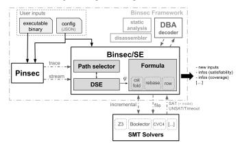
Fig. 1. BINSEC/SE architecture
